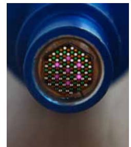
Mixed fiber bundle consisting of UV silica, VIS-NIR silica and CIR fibers to enable remote spectroscopy in 0.2 μm to 6μm spectral range
